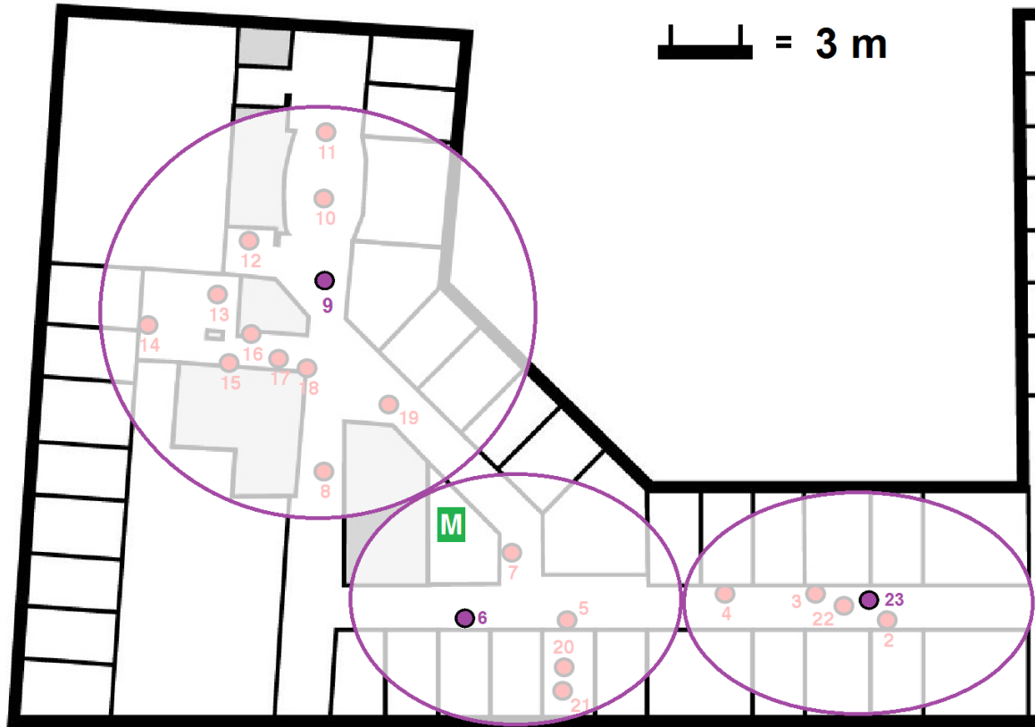
Figure 3.1.: Testbed augmented with JamLab. Nodes 6, 9, and 23 are selected as HandyMotes, and take care of interference (re)generation in their cell.
