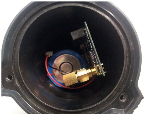
Figure 3.2: A T-mote placed inside a standard FastPrk box.
