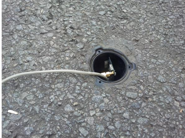
Figure 3.3: A T-mote buried in the tarmac with a debug USB.
