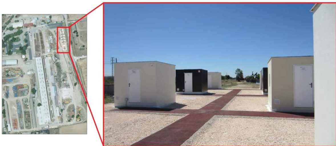
Figure 3.2: Overview of the ACCIONA facility with the buildings used to test insulating materials. Aerial images taken from sigpac.mapa.es .
