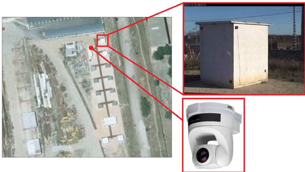
Figure 3.4: The wireless sensor nodes have been installed on the Northernmost building in the facility. A Webcam pointed on the south-west façade of the building has also been installed to monitor and record weather conditions.
